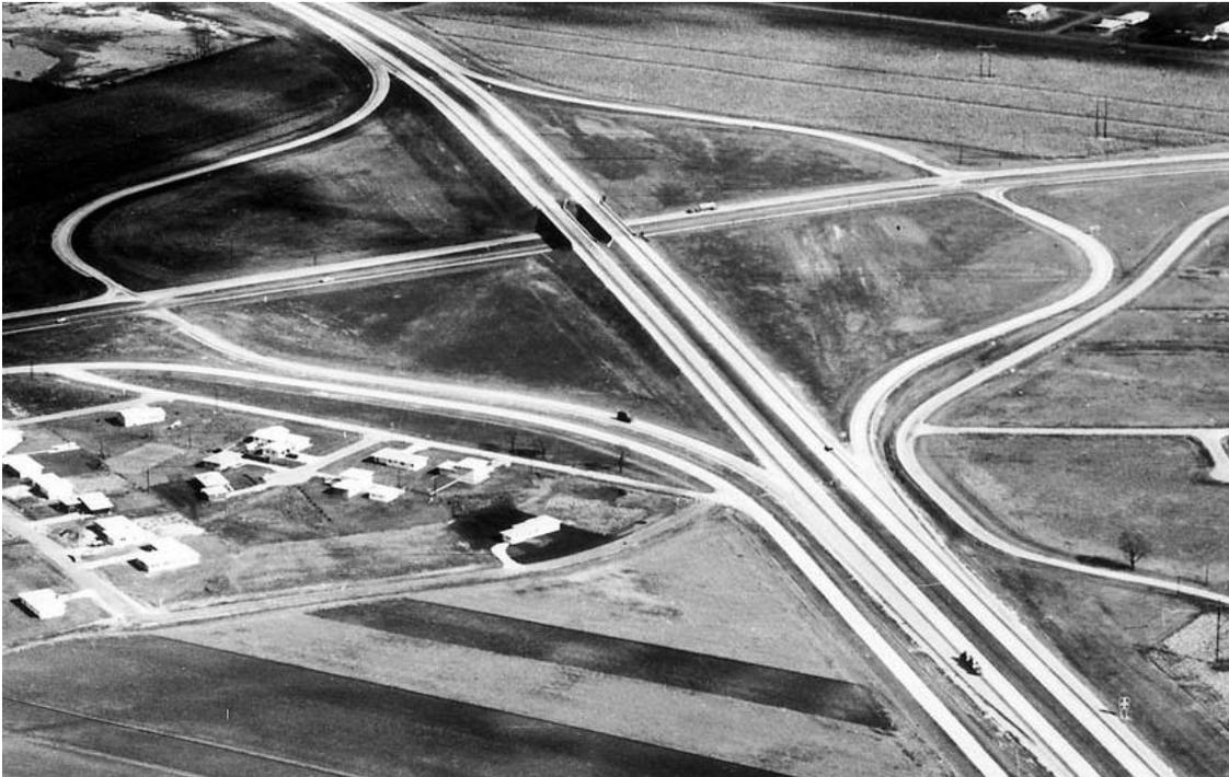
**Exhibit 10-20. Existing Four-Leg Interchange With Diamond Stage Construction**
