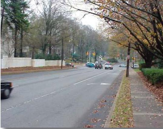
*The image above is a minimal planting strip, providing little buffering from traffic.*
