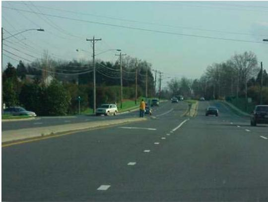
*The situation on the top shows why pedestrian refuges are sometimes needed on multi-lane streets. Below is an example of a simple pedestrian refuge at an intersection crosswalk (photo courtesy of Reid Ewing).*
