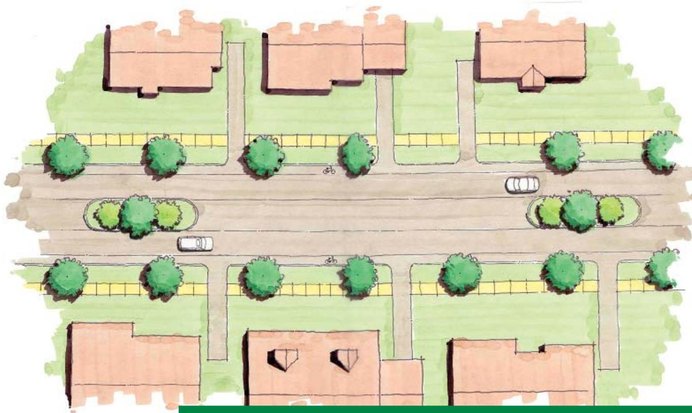
*The 3-lane cross-section with intermittent landscaped islands, not to be confused with 2-lanes and a median. This configuration can also be used for a 5-lane cross-section. The advantages of this configuration include: better access, while removing turning traffic from through lanes; opportunities for pedestrian refuge; lower right-of-way requirements; and an additional source for the “green zone”.*
